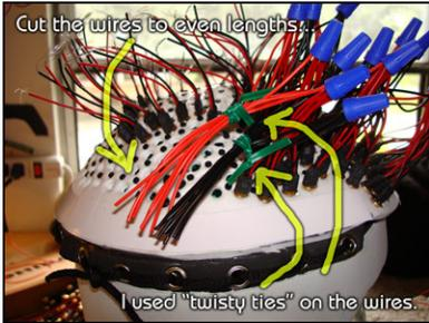
Strip the ends of the wires...
