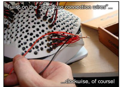
Finally it's time to twist on the wire nuts...
