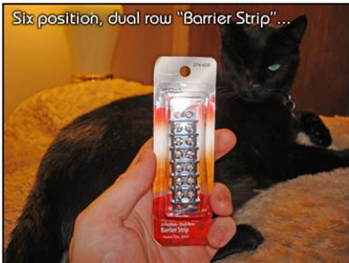
The idea of the "flux capacitor" is to bring the power in from the power supply, split it into three sections, and have plugs on it that each of our three diode zones can plug into.
