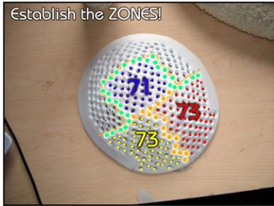
Just make sure you remember which cluster the diodes belong to! In my case, I chose to mark the zones with the diodes of the REAR section, and the diodes of the LEFT section.
